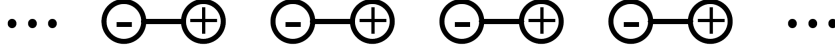
Figure 7.1: As a series of dipoles line up end to end, one can see a current flowing through the line of dipoles as they oscillate back and forth in their polarity. This is similar to how displacement current flows through a capacitor.
